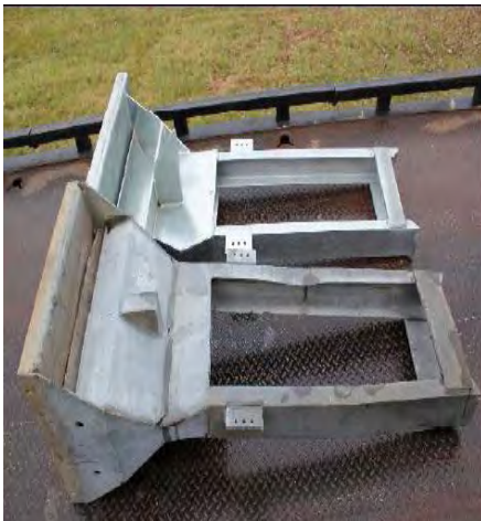
Side view of Trinity ET-2000 (front) and Trinity ET-Plus (back). Photo courtesy Langdon & Emison.
