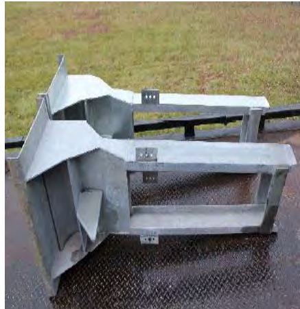
Side view of 5-inch ET-Plus (front) and 4-inch ET-Plus (back). Photo courtesy Langdon & Emison.
