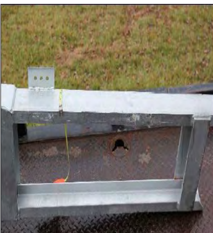
ET-Plus 4-inch guide channel. Photo courtesy Langdon & Emison.
