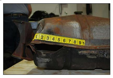
Often there will be no visible "hole" in the seam. However, when the tank is subjected to crash forces, the hydrostatic pressure created inside the tank will cause gasoline to be expelled through very minor cracks in the seam of the tank. The best way to determine if there is a hidden seam split or other compromise of the fuel tank is to inject smoke into the tank under pressure. The smoke will escape from whatever hole or seam split that may exist.
