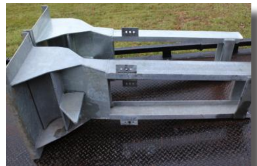
Trinity end terminal defects linked to design changes
