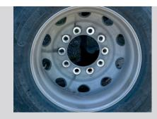
The streaks on this wheel show where the loose lug nuts were, from a recent case of ours.
