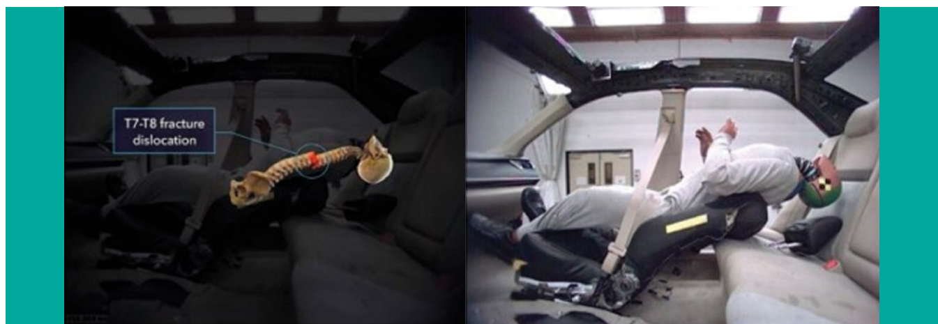
Headrest failure causes spine to hyperextend over the top of the seat. Copyright © 2022 Langdon & Emison Attorneys at Law
