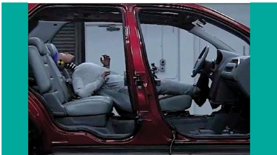
Seat failure causes dangerous contact with rear seat. Copyright © 2022 Langdon & Emison Attorneys at Law
